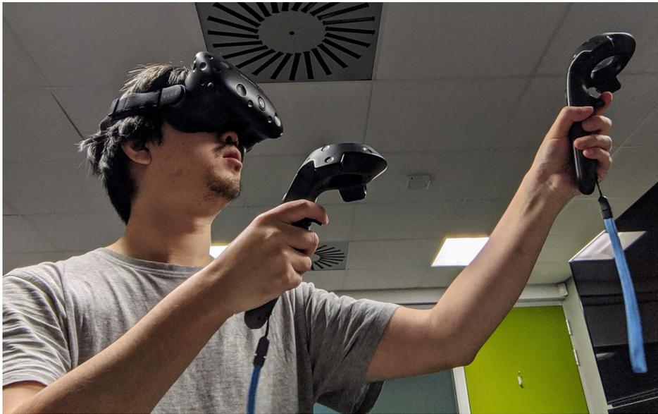
Figure 2.1: An HTC Vive VR headset [32] being used with two tracked handheld controllers.
